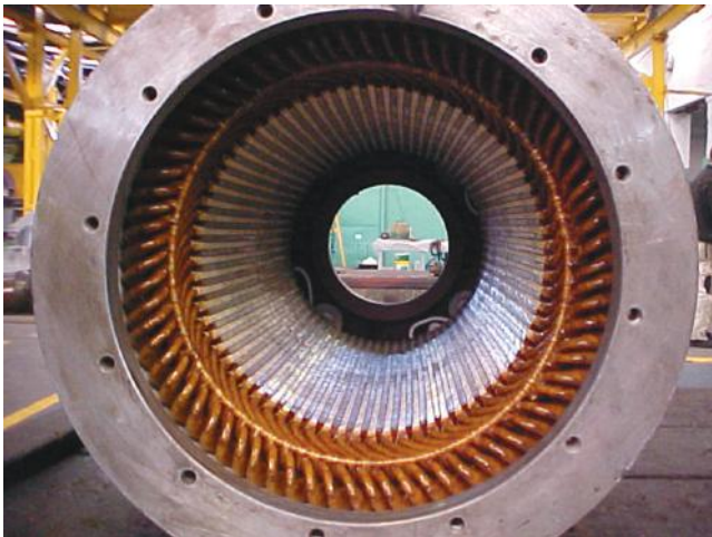
FIGURE 6.13 Medium-sized eight-pole induction machine, with form wound stator coils. (Courtesy of Equacional Motores, Brazil.)
