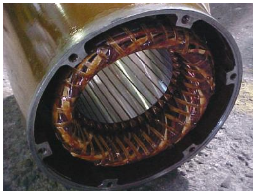
FIGURE 6.18 Random stator winding of a small induction machine. (Courtesy of Equacional Motores, Brazil.)
