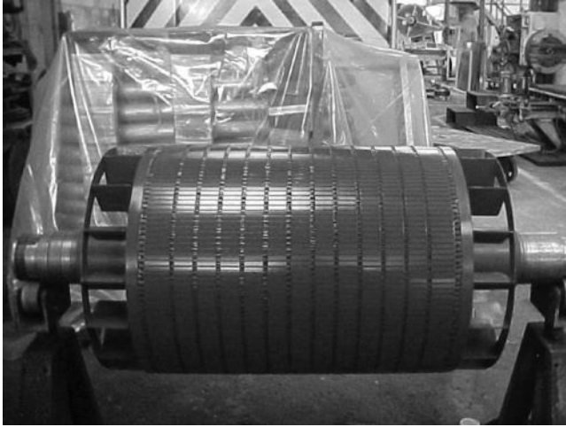
FIGURE 6.4 (See color insert.) Finished squirrel cage for large power induction motor. (Courtesy of Equacional Motores, Brazil.)
