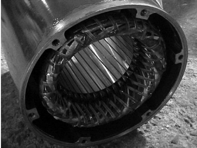
FIGURE 6.18 (See color insert.) Random stator winding of a small induction machine. (Courtesy of Equacional Motores, Brazil.)
